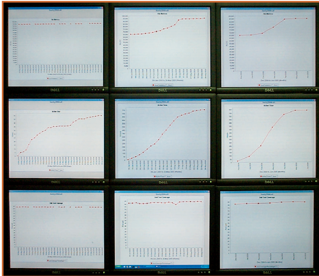
Figure 3. The Telemetry Control Center, which shows one scene consisting of nine telemetry reports. The associated TelemetryViewer software controls the TCC by automatically cycling through a set of scenes at a predefined interval. This telemetry viewer is configured to show a dozen separate scenes, each displayed for two minutes.
