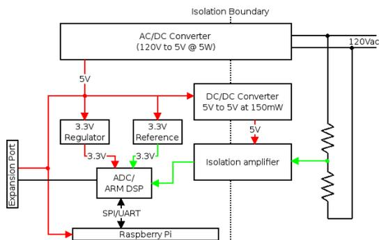
(a) OPQ Box Block Diagram. The power path is in red, signal path is in green and the digital IO is in black.
